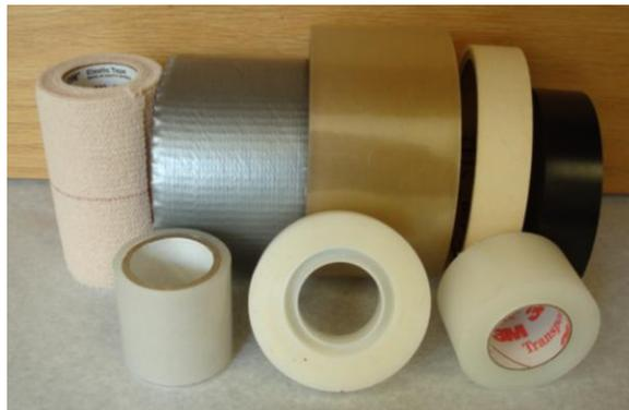
Types of tape compared in this study. Back, left to right: elastic, duct, packing, masking, and electrical tapes. Front, left to right: lifting, Scotch<sup>®</sup>, and surgical tapes. For interpretation of the references to color in this and all other figures, the reader is referred to the electronic version of this thesis.
