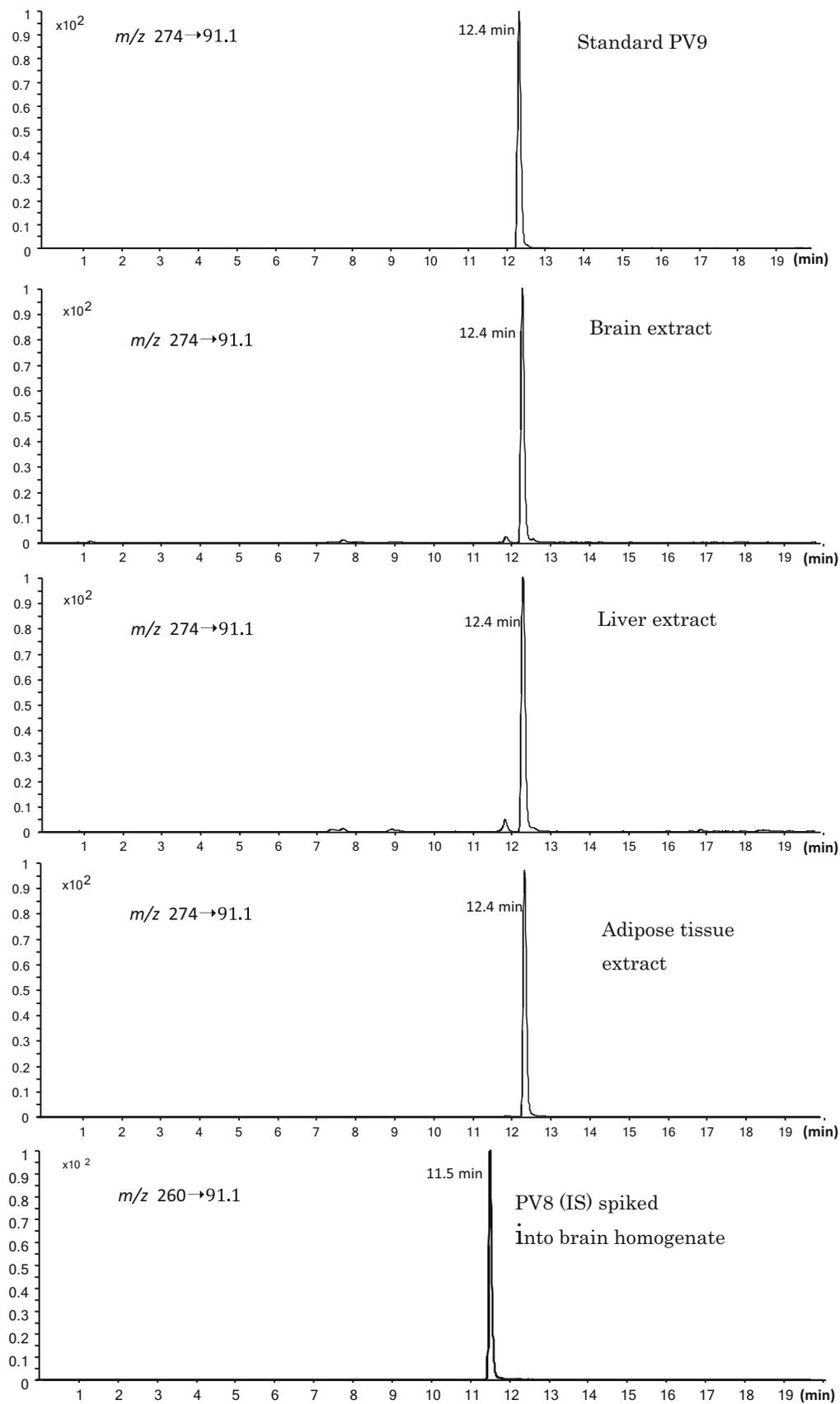
**Fig. 2** Selected reaction monitoring chromatograms for the reference standard PV9 and the extracts of the postmortem brain, liver, and adipose tissue and for PV8 (internal standard) spiked into the brain tissue, recorded by LC–MS–MS
